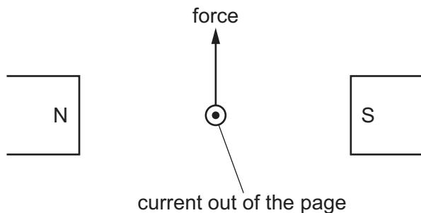
Both the direction of the current and the poles of the magnet are now reversed.
